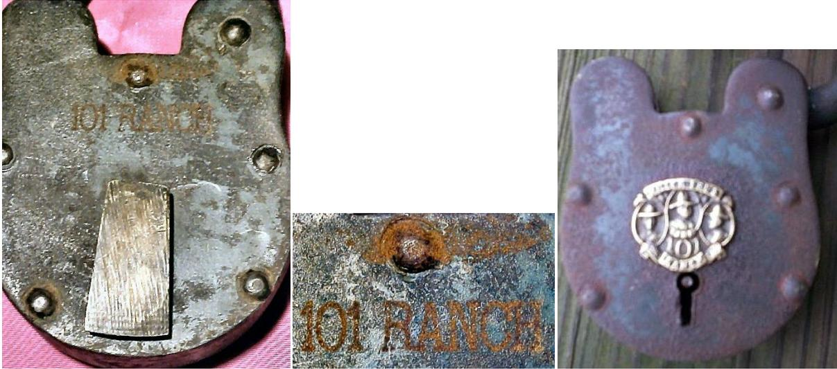
**The lettering on the first lock has been etched into the metal. The second lock has an emblem that has been soldered to the front of the lock.**
